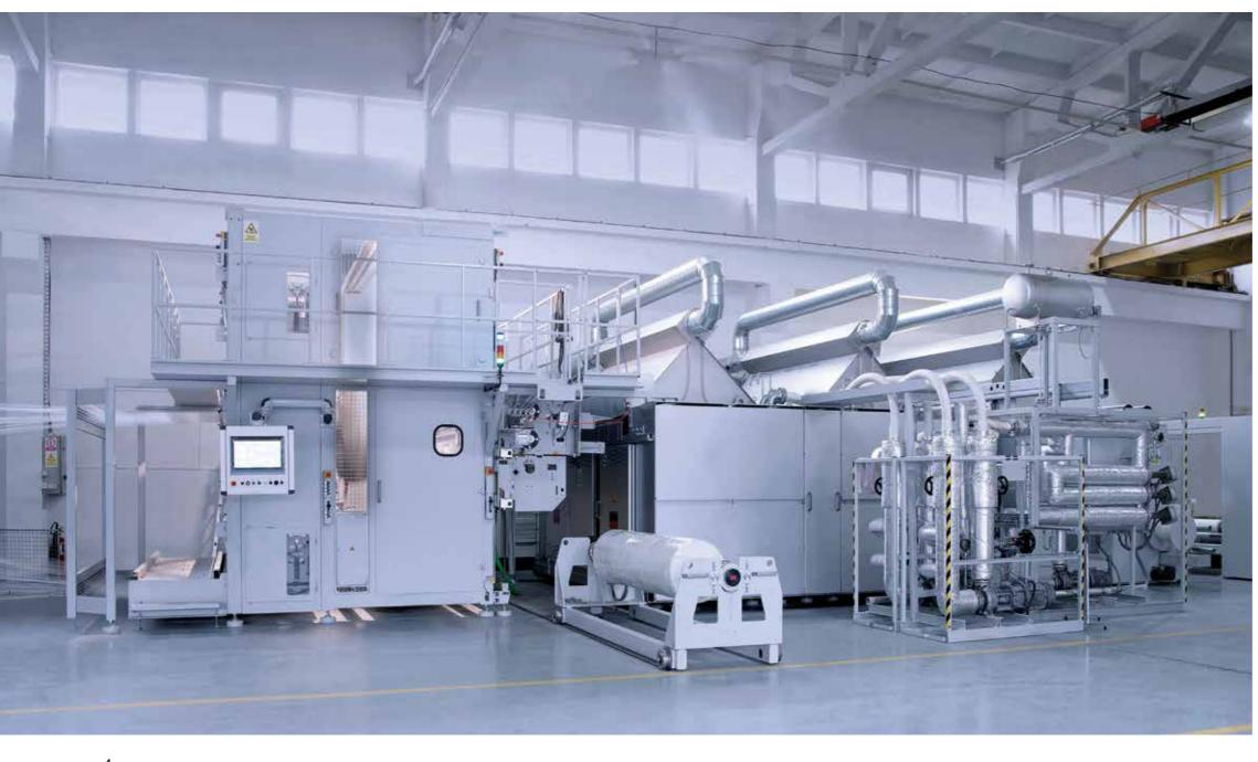
The TURBOTEX is a machine for the production of scrim fabrics.
